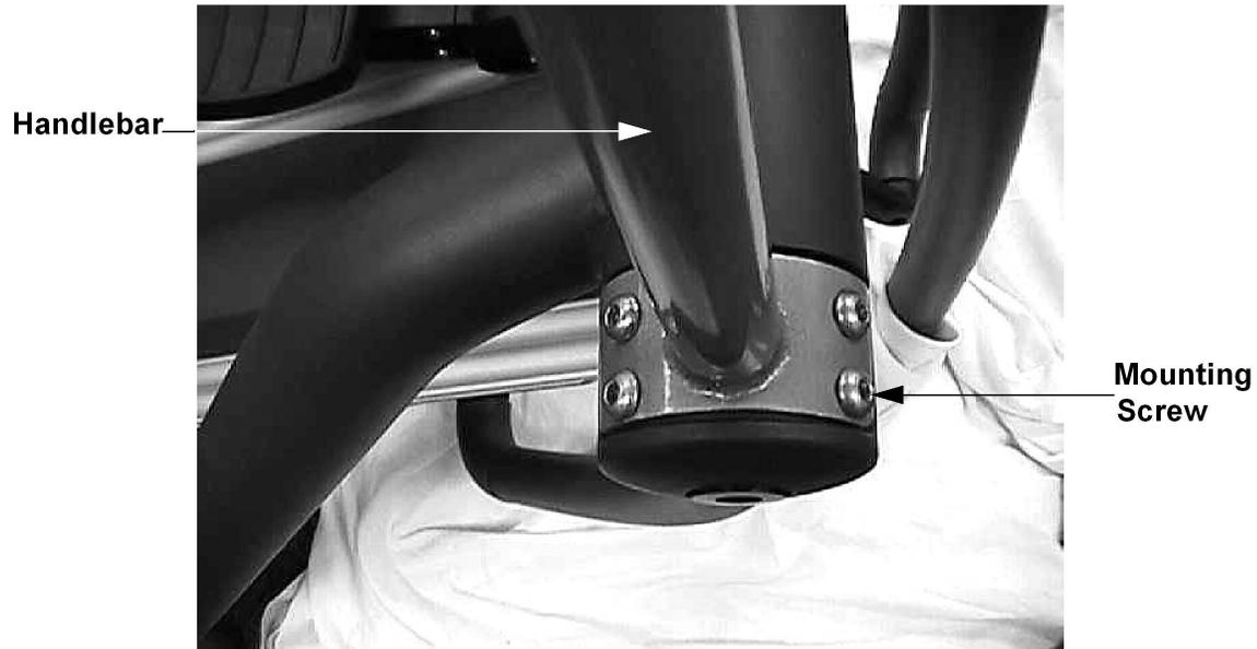
3. Set the replacement handlebar in its mounting position. Hand start the four mounting screws. Center the handlebar in the indented area of the upper pivot arm. Torque the four mounting screws to 300 inch pounds.
